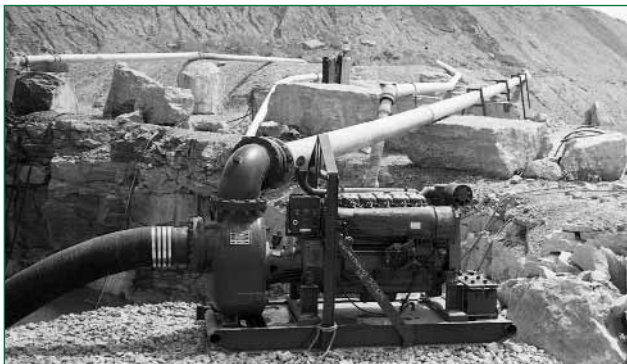
A self-priming 12 in. trash pump with air-cooled diesel power on skid.
