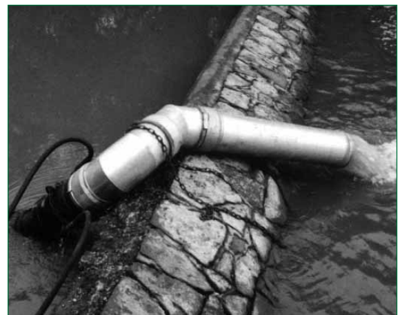
A 12 in. mixed flow hydraulic submersible pump.
