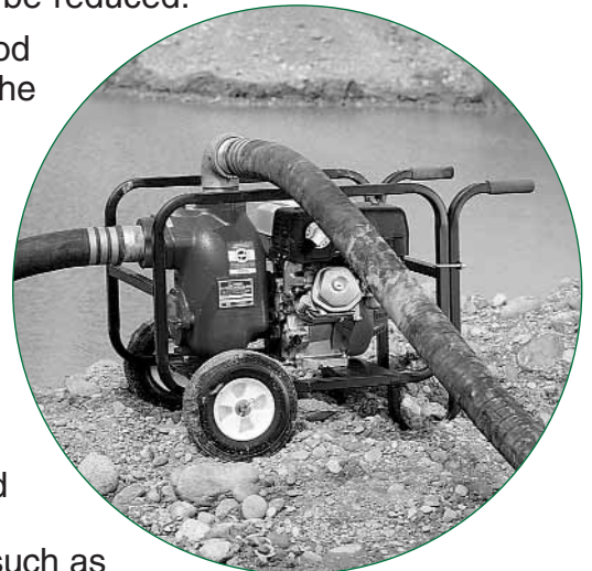
A 3 in. self-priming trash pump with air-cooled gas power on site cart.
