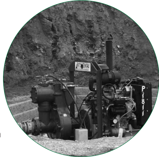
A 6 in. vac assisted centrifugal trash pump.
